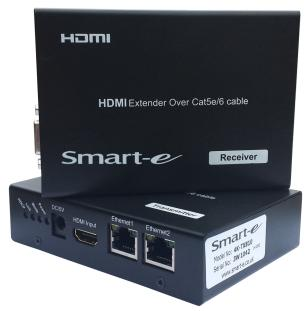
The **4K-909** is a transmitter and receiver pair designed to extend HDMI, DVI or DisplayPort, together with reverse IR, Ethernet and bidirectional RS232 signals over a single twisted pair CAT 5e-8 cable. The units use HDbaseT technology to extend 12 bit Deep Colour 3D, 4K and 2K resolutions together with 1080p @60Hz
