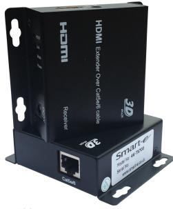
The **4K-700** is a transmitter and receiver pair designed to extend HDMI, DVI or DisplayPort, together with IR signals over a single twisted pair CAT 5e-8 cable. The units use HDbaseT Lite technology to extend 12 bit Deep Colour 3D, 4K and 2K resolutions together with 1080p @60Hz
